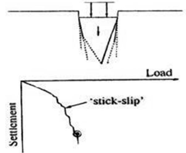
Punching Shear Failure
